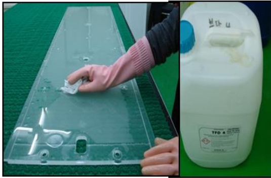
CLEANING 1 (油分除去)
